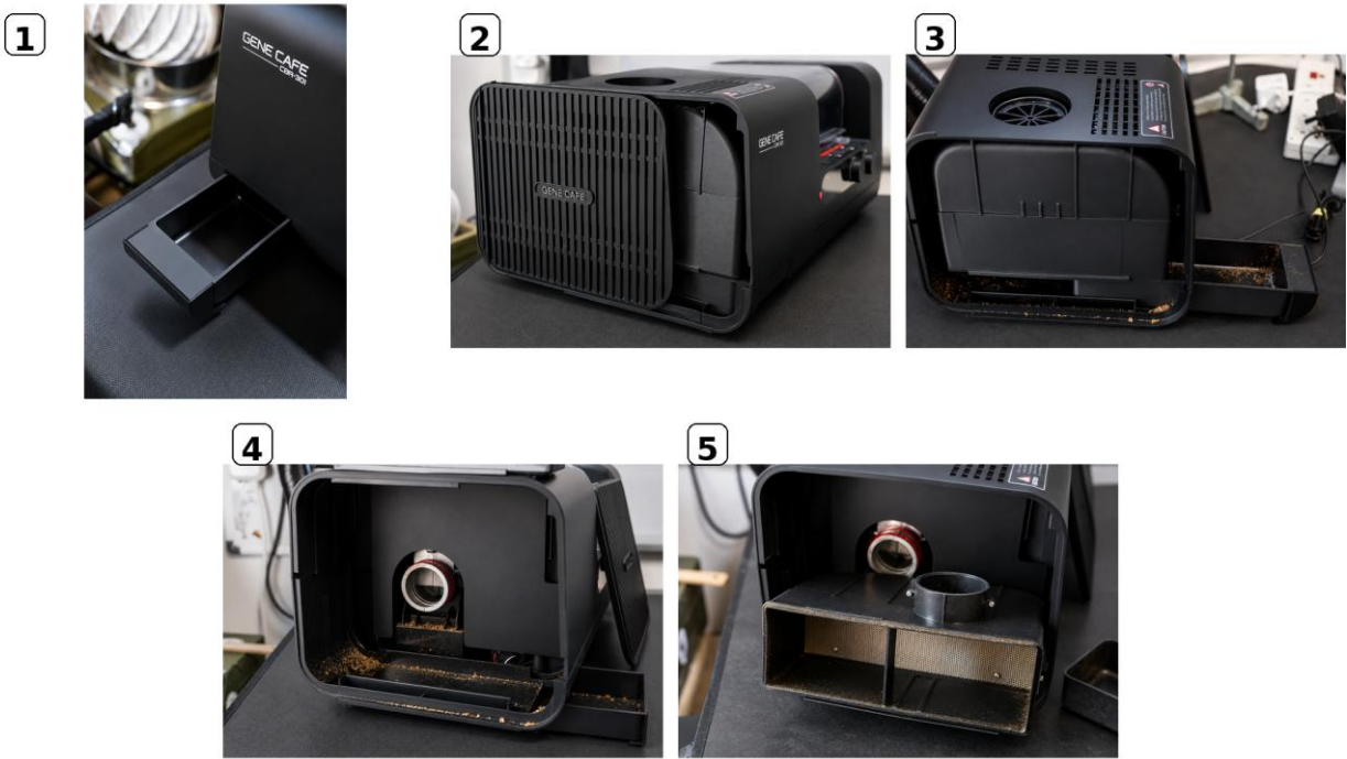
Figure 9. Chaff-box removal and cleaning sequence. The numbered photographs show the left-side chaff tray and cover, the chaff-box body, the exposed air outlet after removal, and the mesh area that must be kept clear. Follow the written procedure and reassemble all parts securely before the next roast.
