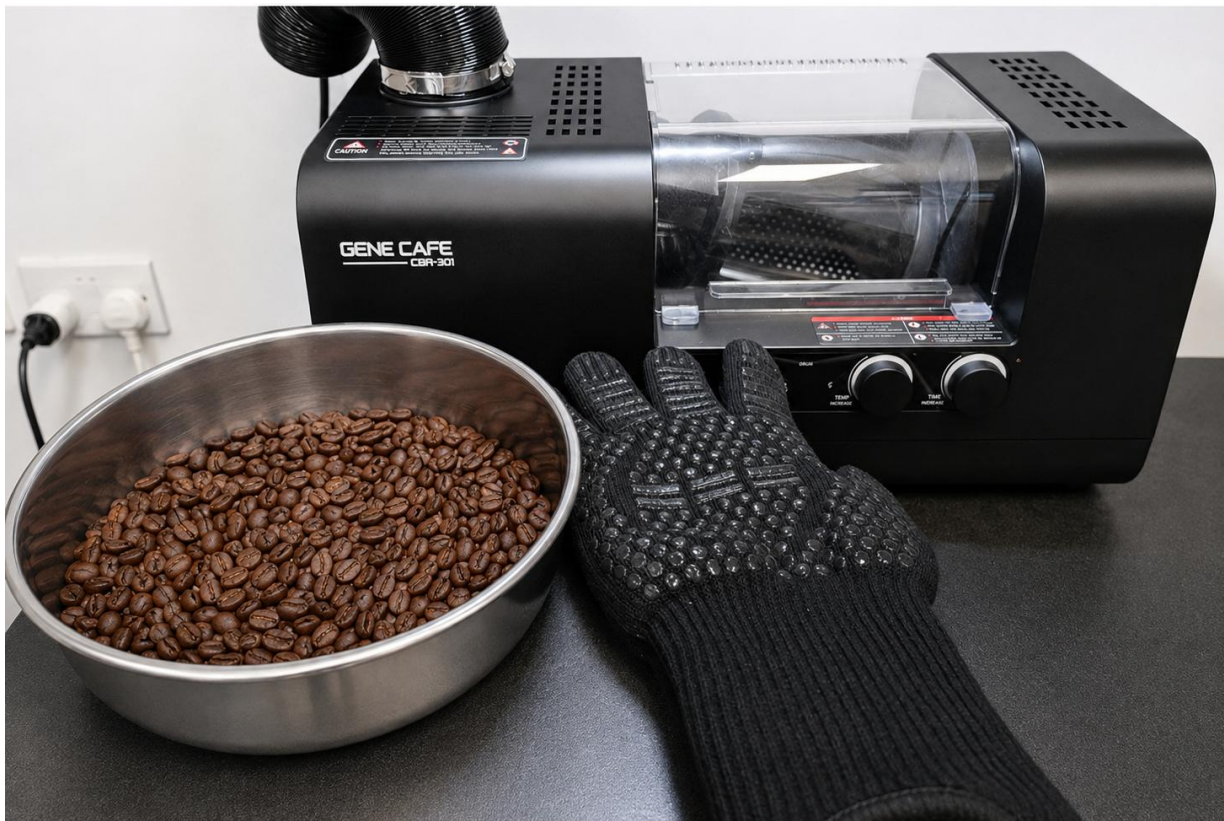
Figure 6. External bean-cooling setup. Have the external cooler and properly fitting heat-resistant gloves ready before removing the hot chamber; follow the complete procedure above.
