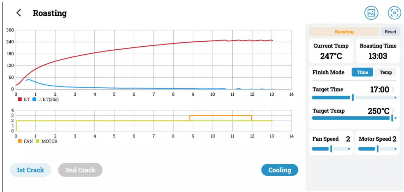
Figure 3. Gene Café app during an active roast. The upper graph plots ET and \Delta ET as high-level references, while the lower graph records fan and motor levels. The right-hand panel shows elapsed time, displayed temperature and the current settings. The 1st Crack and 2nd Crack buttons add manual markers, and Cooling sends a command to the roaster. The graph records and compares the roast; it does not instruct the machine to follow a profile.
