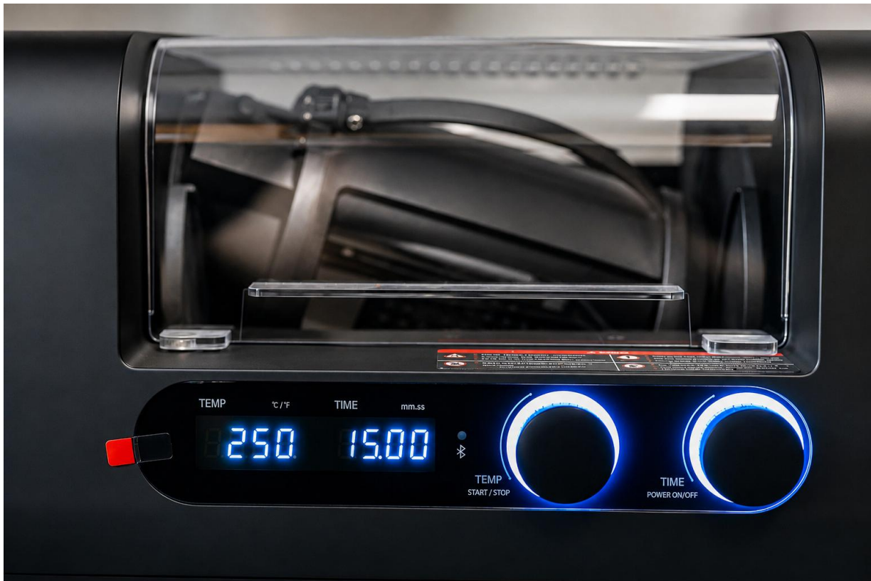
Figure 2. Front-panel controls and display. TEMP sets the target temperature and starts roasting or cooling; TIME powers the machine and sets the planned duration.
